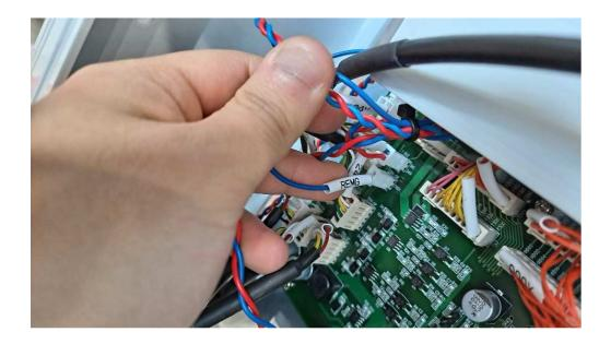
8. IMM Interlock I.O PC 18 will turn on and off (This is new style interface board, old style might have relay)
