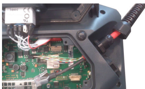
Fig.5-5: Inserting connection cable
