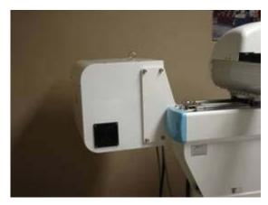
( Control box need to be mounted at the end of robot beam body : wiring harness need to be tied up with cable tie ), also need to assemble cover ( Kick front and Back )
