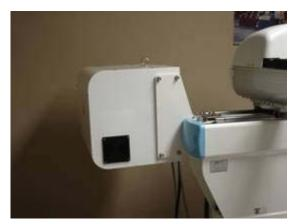
( Control box need to be mounted at the end of robot beam body : wiring harness need to be tied up with cable tie ), also need to assemble cover ( Kick front and Back )
